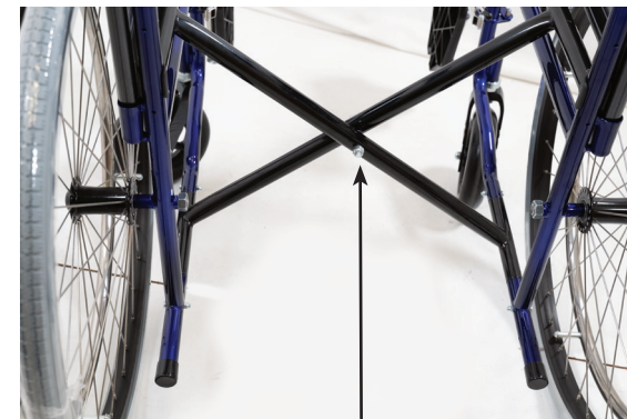
Cross-brace centre bolt
