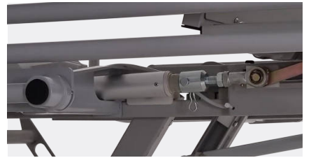
Step 18: Finalise refitting the actuator.
