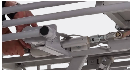
Step 17: Refitting the actuator.
